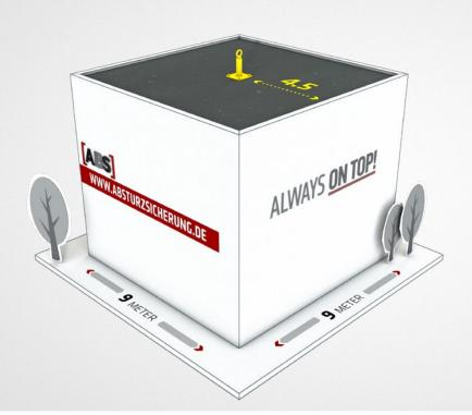
In the illustrated example, a single ABS-Lock anchorage point is located 4.5 meters from the edge of the roof.
