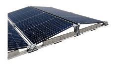
Application Flat Roofs Simply insert paving stones (bricks) into the floor rails provided as ballast material. This keeps your ABS BASE Weight firmly in place. The robust design of this highly weather-resistant aluminium substructure and the simple installation process guarantee that your solar panels can be installed safely.
